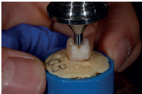
Fig. 1: Insert with a 3 mm spherical tip.
