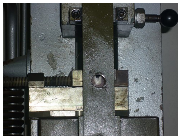
Fig. 3: Specimen placed in a press on the universal mechanical testing machine to undergo the shear test.
