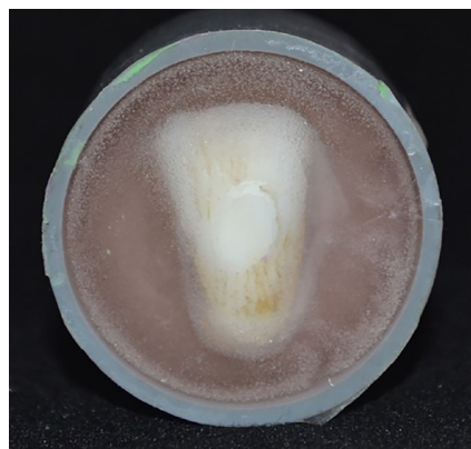
Fig. 1: Specimen dipped in acrylic resin, with the enamel surface free for adhesion.
