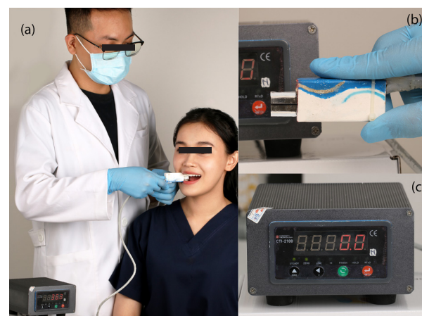
Fig. 1: (a) Biteforce Meter BFM 4th generation, Vietnam, certificate of calibration number SG19-0390 by Sai Gon technology center for measurement and calibration; (b) Biteforce Meter BFM 4th generation biting transducer; (c) Biteforce Meter BFM 4th generation screen display.
