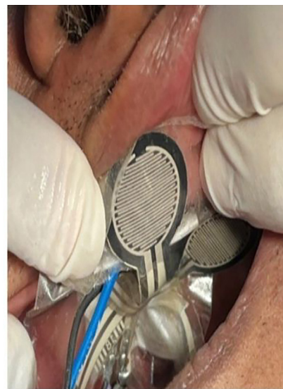
Fig. 1: (a) An integrated system with tongue pressure (S1, S2, S3, S4, S5) and bite force measuring sensors (B1, B2, B3, B4, B5) and (b) Placement of pressure sensors against the palate for recording tongue pressure.
