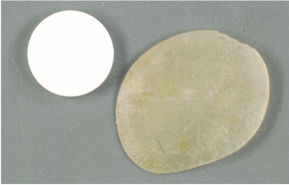
Fig. 2. Ivory cross-section 1 cm in diameter and 300 \mu m thick next to a calcium phosphate pellet used to calibrate the photographs.
